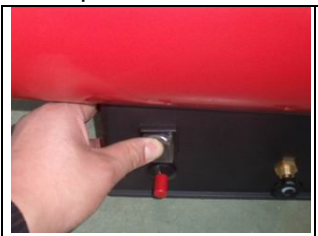
put the power switch at position“1”
